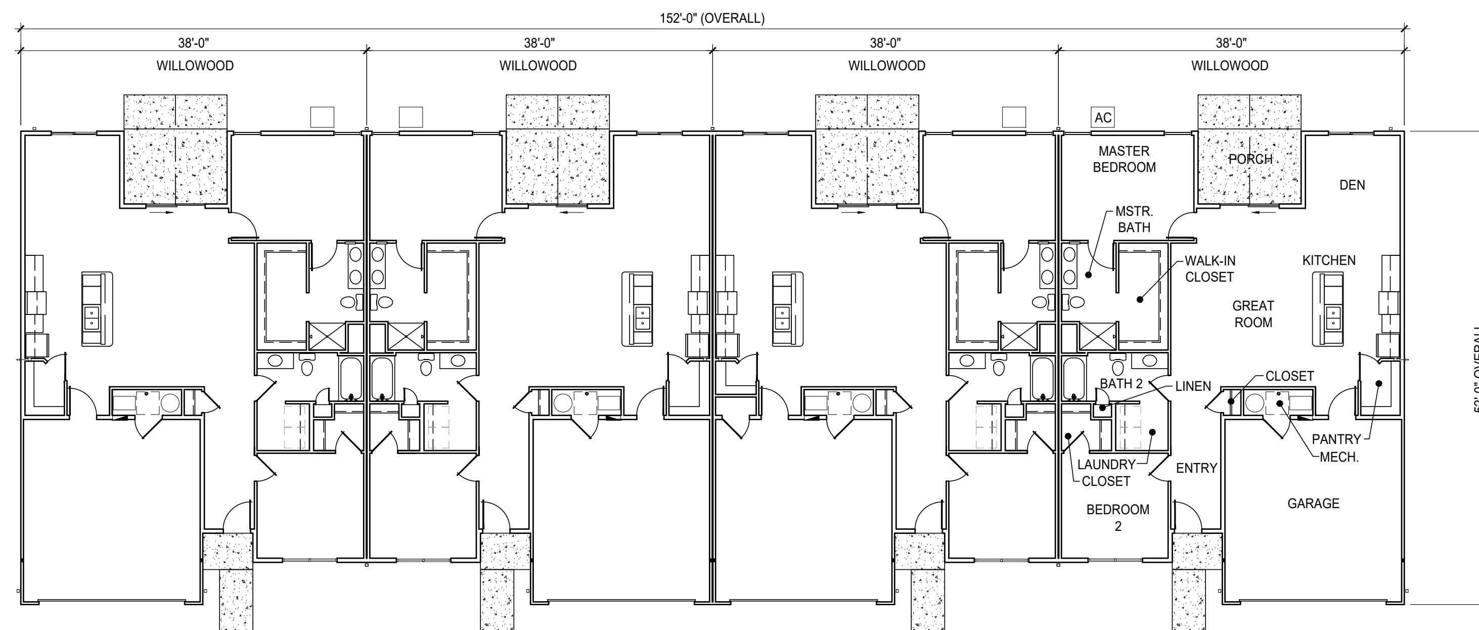
OVERALL FLOOR PLAN WILLOWOOD SCALE: 3/32" = 1'-0"
